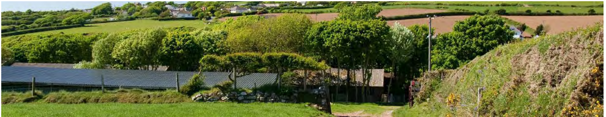
Above: The siting of farm buildings within a hollow and adjacent to well established planting softens the impact of the development, as does the use of a dark matt roof colour
