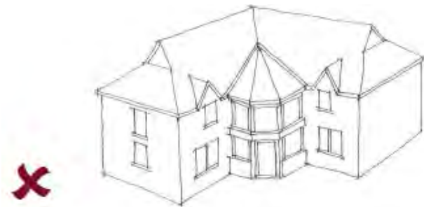
Use of various complicated roof forms create a visually disjointed roofscape
